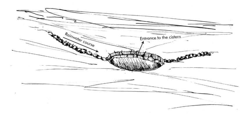
Figure 16: Drawing of a naqaba (cistern)
